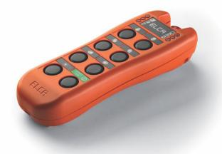
EVO is a brand new radio remote control, developed and produced by ELCA in full compliance with applicable laws\* for machines and industrial lifting and handling. It consists of 6 double step push buttons, 1 programmable function button, Start and mushroom STOP.
